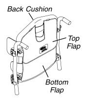
FIGURE 2 - INSTALLING/REMOVING CUSHIONS
